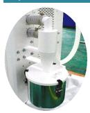
The device is to remove excess dust on the conveying line with the cyclone method and equipped with a dust collector tank as a dust reservoir with latch lock so it is easy to open the dust tank.
